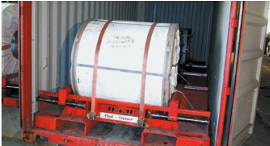
Steel coil secured on a Coil-Tainer cradle
