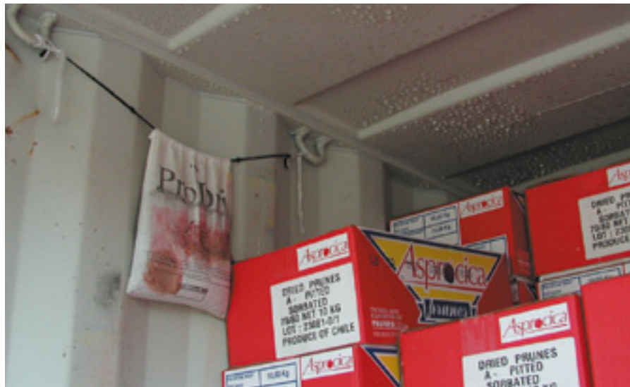
Condensation water on roof, dry bag already completely soaked
