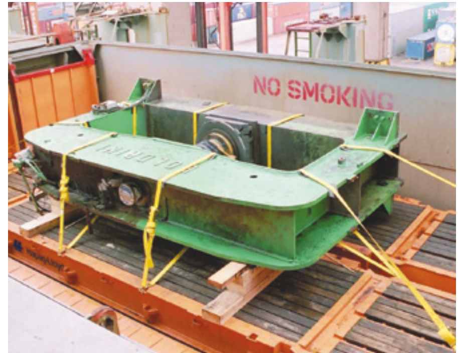
The press is placed on two flatracks. Sturdy square timbers are put under the press on the flatracks to distribute the weight and prevent damage to the cargo or to the flatrack. Nylon belts have been used for lashing
