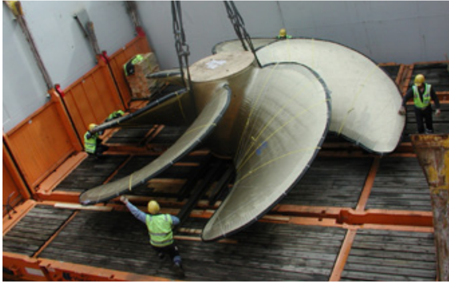
Loading a large ship propeller weighing 80t. The propeller has a very small contact area, so robust steel bedding is applied. Steel wires or nylon straps will be used for securing
