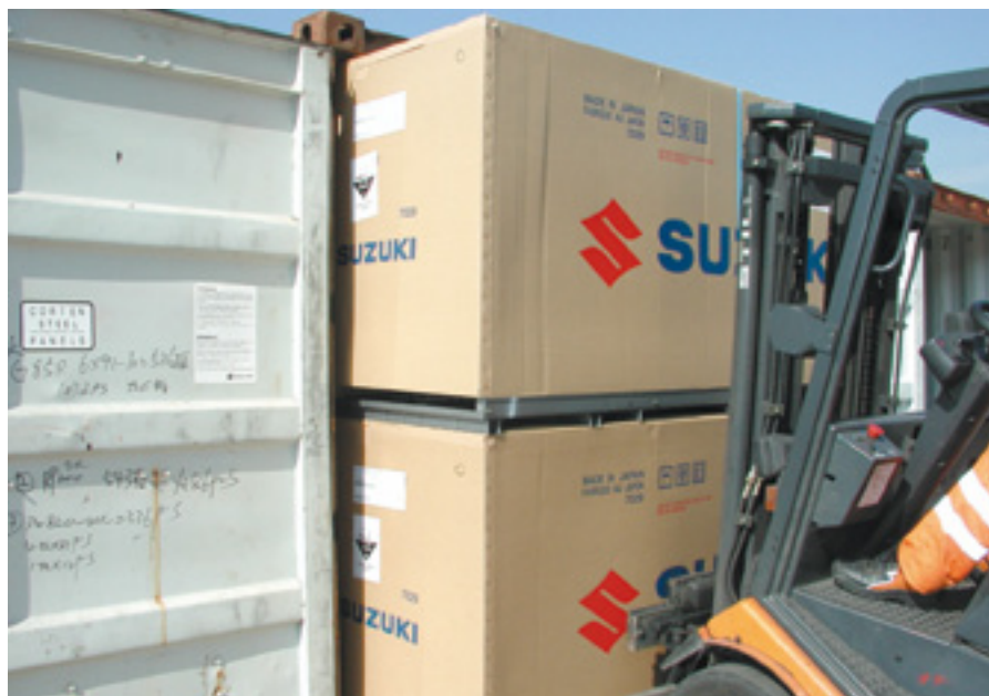
The size and structure of the packing for the motorcycles correspond with container dimensions
