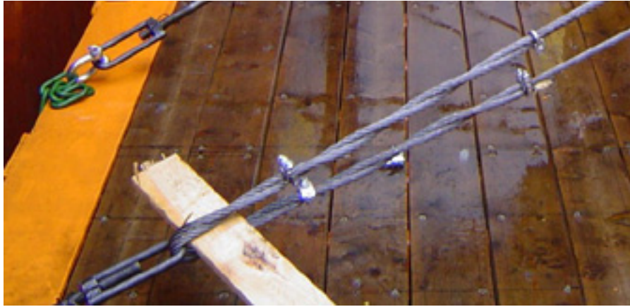
Correct lashing arrangement. The steel wire is twisted to increase the friction
